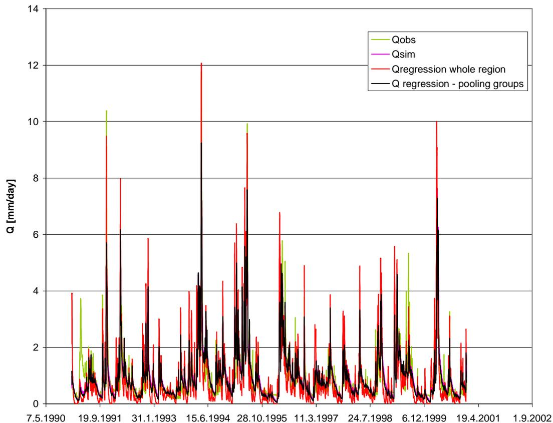
Fig. 3 Observed runoff, runoff obtained by model calibration and runoff obtained by regional regression formulae in Čierny Hron sub-catchment (7045).
