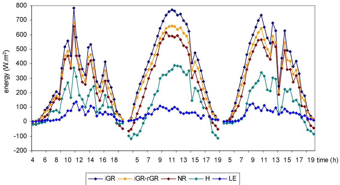
Fig.3. The proportional course of net radiation (red line), the sum of the sensible and the latent heat flux (violet line), the sensible heat flux (orange line), latent heat flux (green line) and the reflected global radiation (blue line) from the incident global radiation observed above the spruce stand in the EESS at Bílý Kříž during 26<sup>th</sup>-28<sup>th</sup> May 2000 (all line were smooth using the moving average 5).
