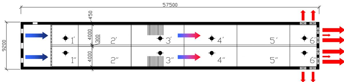
Fig. 1 Ground layout, measurement places in pens (1, 3, 4, 6) and air movement in stable
