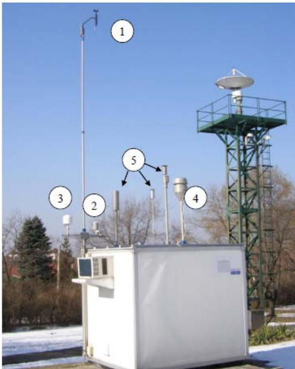
**Figure 3.** Example of urban monitoring station; meteorological sensors: wind (1), temperature (2), global solar radiation (3), precipitation (4), air quality (5) gas and aerosol samplers.
