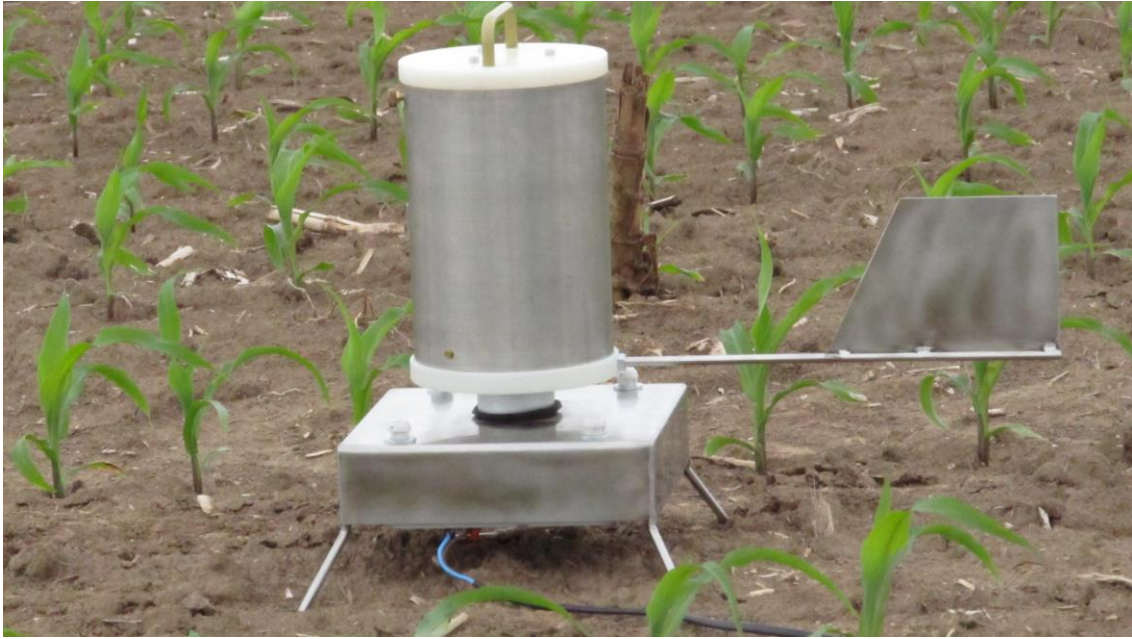
Fig. 9 Deflameter with active trap soil particles and time recording (Krmelová et al., 2012)
