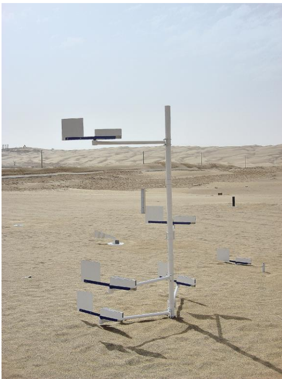
Fig. 4 Big Spring Number Eight sampler (Zobeck et al., 2003)
