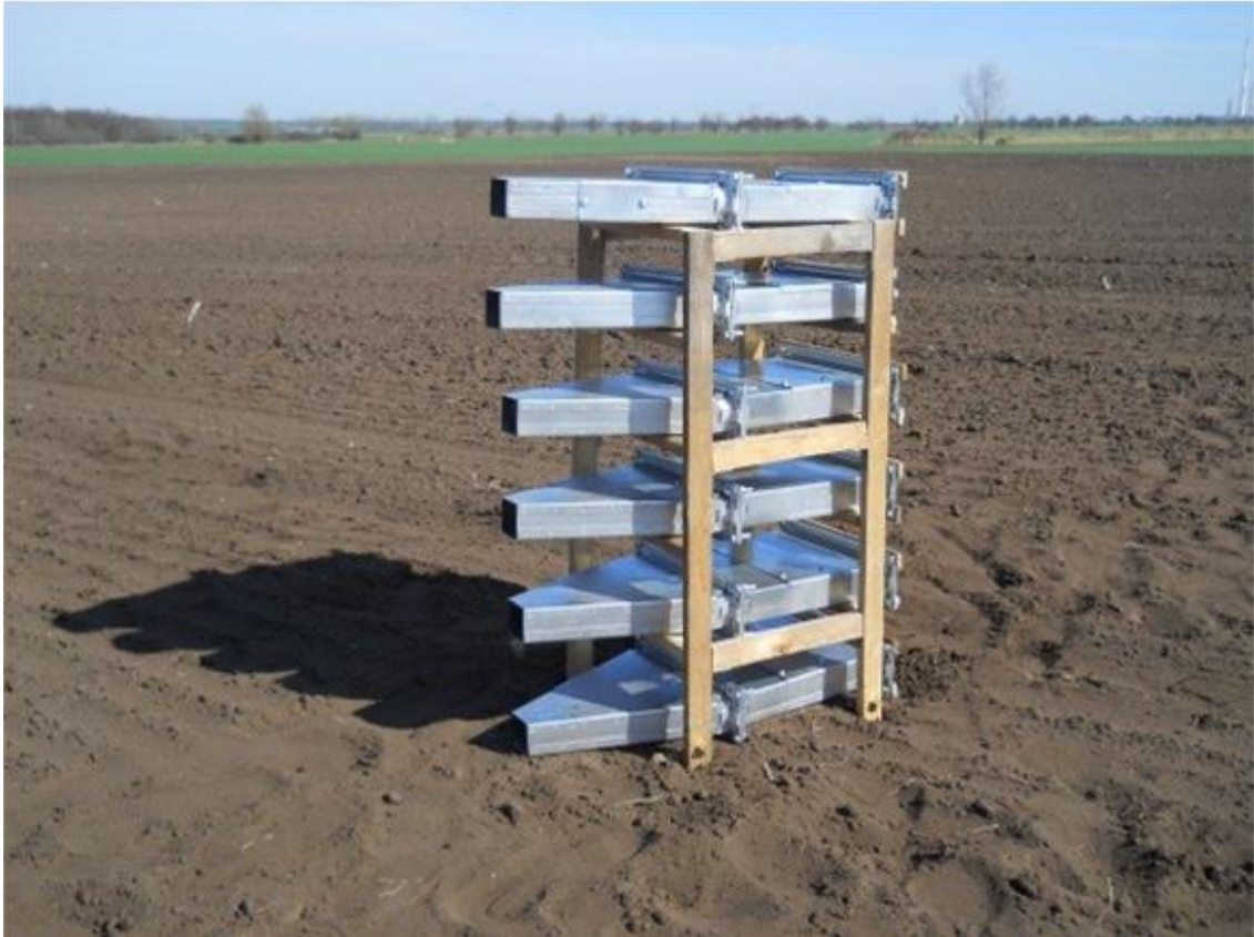
Fig. 10 Soil particle catcher devices (Lackóová et al., 2013)
