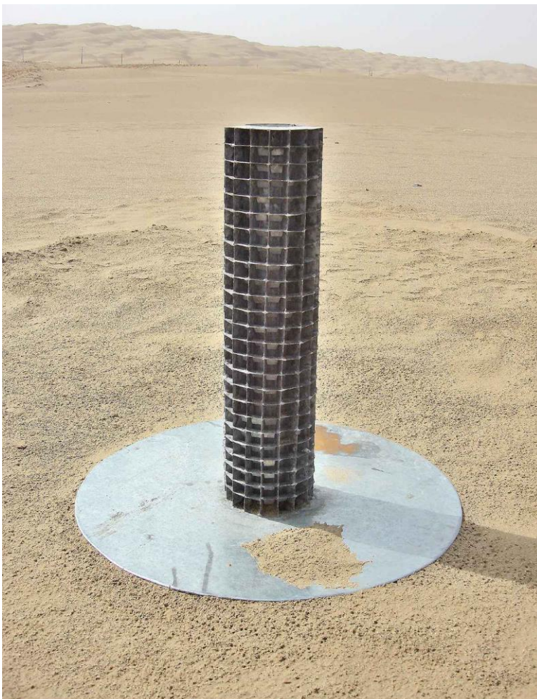
Fig. 1 Bagnold collector ( www.sensit.com )
