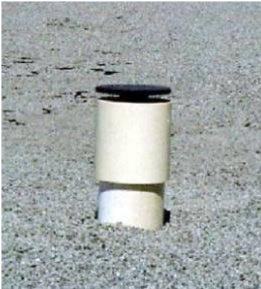
Fig. 2 Cox sand catcher ( www.sensit.com )
